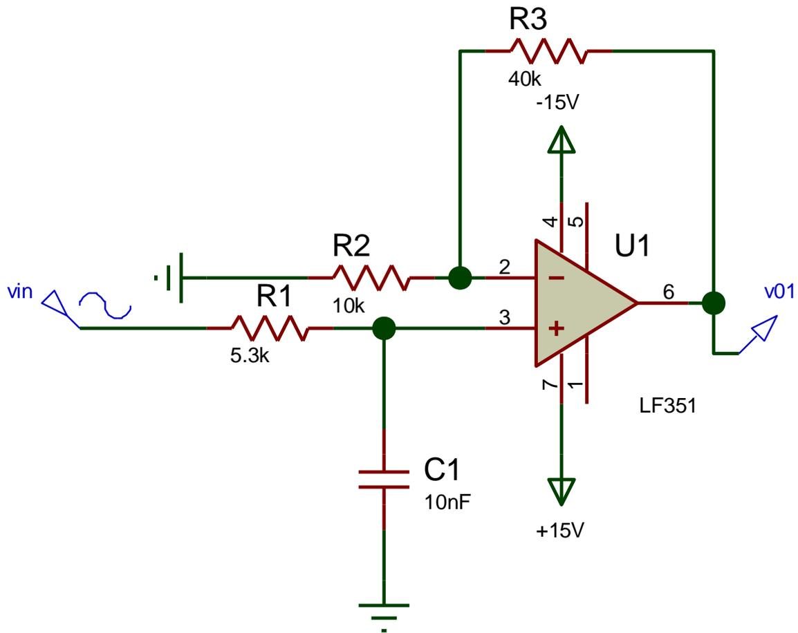
$$f_t = 3000 \text{ [Hz]} \quad \text{pongo} \quad C_1 = 10 \text{ [nF]} \quad \ggggg \quad R_1 = 1 / (2\pi \cdot 3.000 \cdot 10^{-8}) = 5,3 \text{ [K}\Omega\text{]}$$
