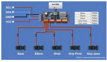
The I2C connections are made to one of the connectors on the end of the PCA9685, either connector will work.
