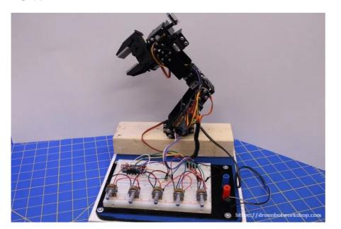
The brackets and supports for the arm are constructed from black anodized aluminum which makes for a strong support.
