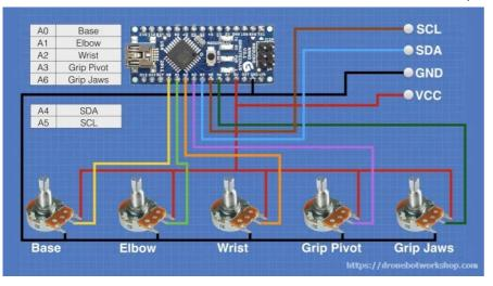
The "Arduino section" of our wiring diagram has the Nano and the 5 potentiometers. The controls are wired with one side to ground and the other side to 5 volts, obtained from the Arduino Nano.
