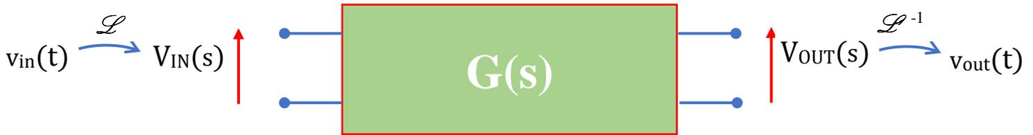
$$V_{OUT}(s) = G(s) \cdot V_{IN}(s)$$
