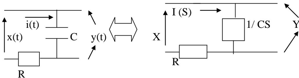
$$\begin{aligned} \text{f.d.t} = F(j\omega) &= Y / X = (1 / j\omega C) I / (R + 1 / j\omega C) I = \\ &= 1 / 1 + j\omega CR \end{aligned}$$
