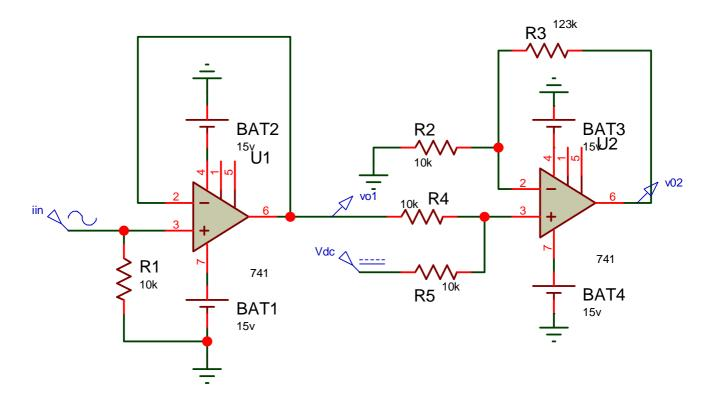
$$v_{01}(t) = i_{in}(t) * Rf = 0.75 \sin(2\pi 1000t) + 2.25$$
