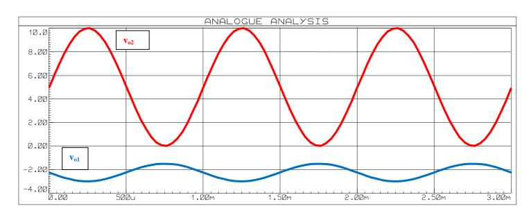
$$v_{01}(t) = \text{-} \ i_{in}(t) * Rf = \text{-} \ 0.75 \ sin(2\pi 1000t) - 2.25 \quad [V] \\ \text{Vdc} = \text{1.5} \ [V]$$
