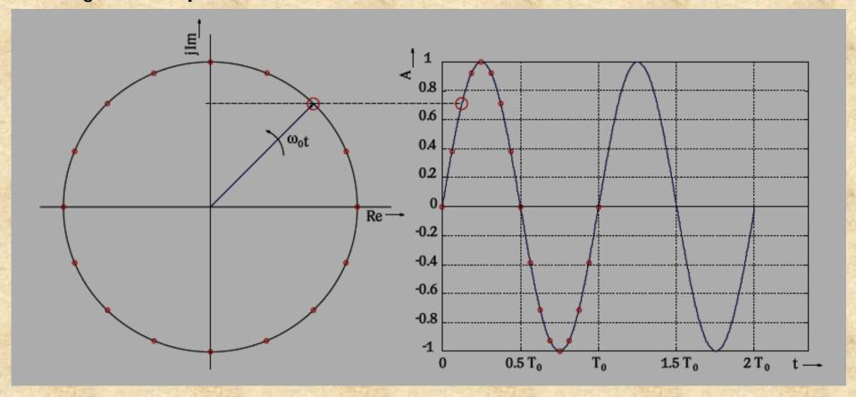
$$V(t) = 1*\sin(\omega_o t) \quad dove \quad \omega_o t = 2\pi/T_o \cdot t = 2\pi f_0 \cdot t$$
