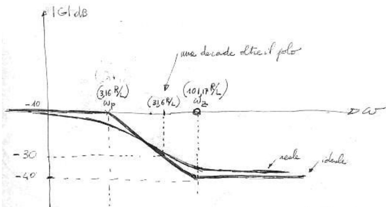
$$|G| = \frac{\sqrt{R^2(R_1+R_2)^2 + (\omega L R)^2}}{\sqrt{(RR_1+RR_2+R_1R_2)^2 + [\omega L(R_1+R_2)]^2}}$$
