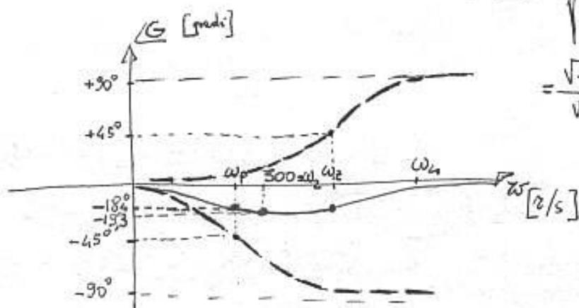
$$|G(j\omega_2)| = \frac{\sqrt{1 + \left(\frac{1}{R_2 C} - \frac{C R_2}{R_1 + R_2}\right)^2}}{\sqrt{1 + \left(\frac{1}{R_2 C} + \frac{R_1 + R_2}{R_2 C}\right)^2}} = \frac{\sqrt{2}}{\sqrt{1+4}} = \frac{\sqrt{2}}{\sqrt{5}} \Rightarrow [-4 \text{ dB}] [0,63]$$
