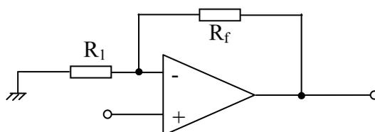
$$A = 1 + R_f/R_1 \quad R_f/R_1 = 4$$
